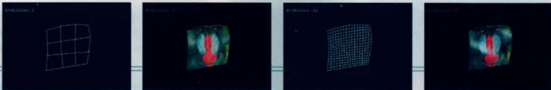
This demonstration of curved patches, using software written by Argonaut, illustrates how increasing the number of small surfaces incrementally can change the smoothness of the shading on the final textured image to create a high quality image
